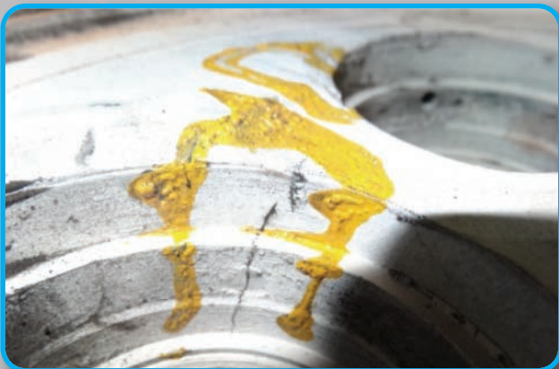
Cracked valve seat pocket
