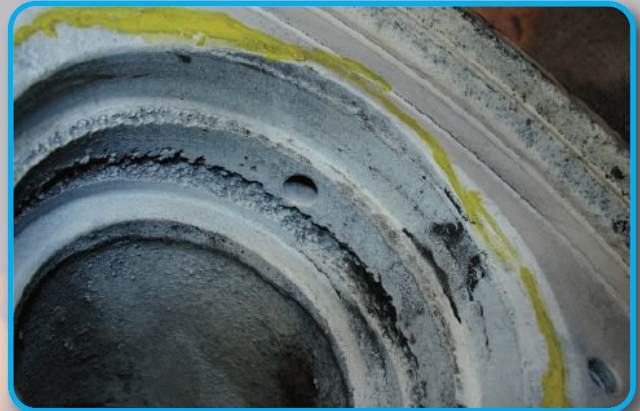
Heavy corrosion to wall of valve seat pocket
