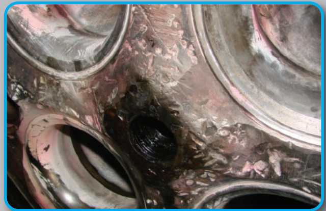
Severe mechanical damage to combustion face
