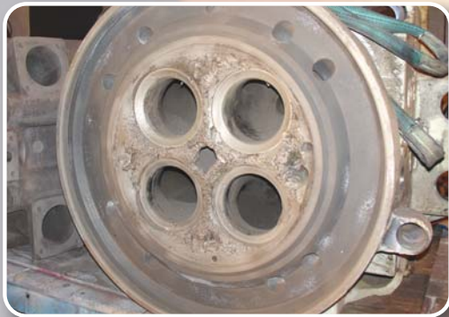
Wartsila 46 - Impact damage to flame face.
