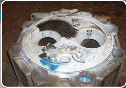
Hanshin 46 - Lifted flame plate.
