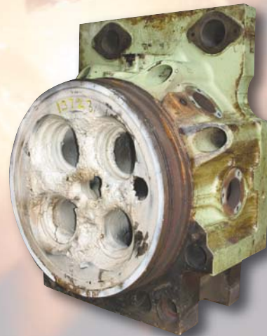
MAN48/60 - Extensive mechanical damage.
