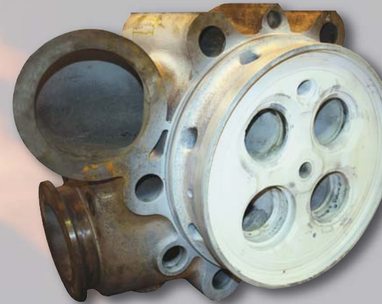
MaK M32 - Exhaust valve seat pocket eroded beyond manufacturers maximum oversize.
