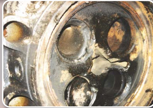
Stork TM410 - Dropped valve with injector port damage.
