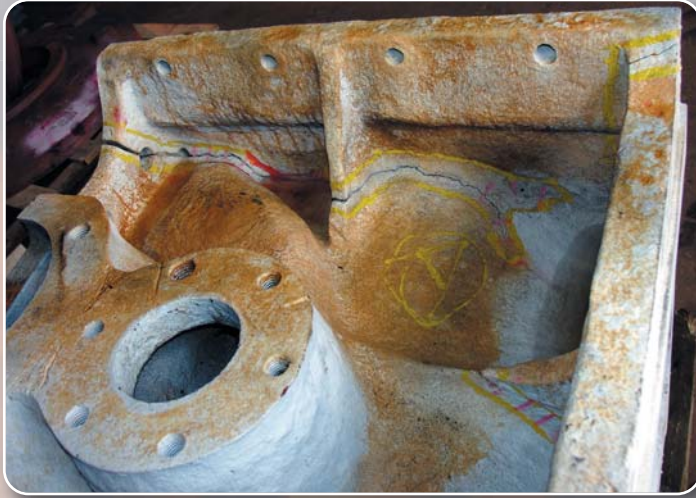
Block received in cracked and distressed condition. Cracks highlighted by M.P.I. crack detection.
