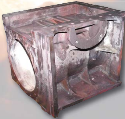
Gas Fusion welded block after the pre-heat procedure fully stress relieved and before sand blasting.
