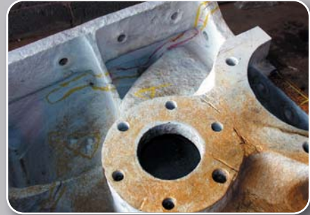
Block received in cracked and distressed condition. Cracks highlighted by M.P.I. crack detection.
