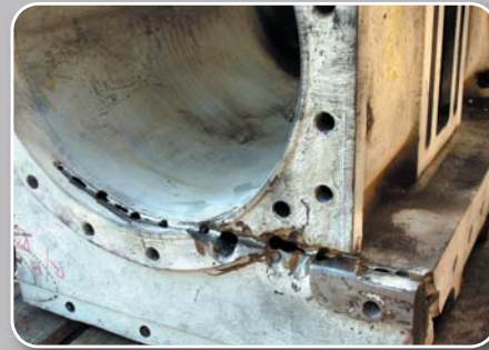
Gas Fusion welded block after the pre-heat procedure fully stress relieved and before sand blasting.
