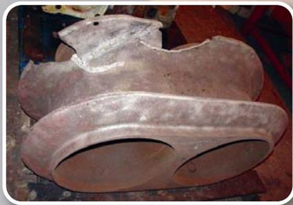
This double chimney stack casting was broken and had been poorly repaired. We replaced the missing sections of the casting, blending the new metal into the original and gas fusion welded the cracks. The stack is now serviceable again.
