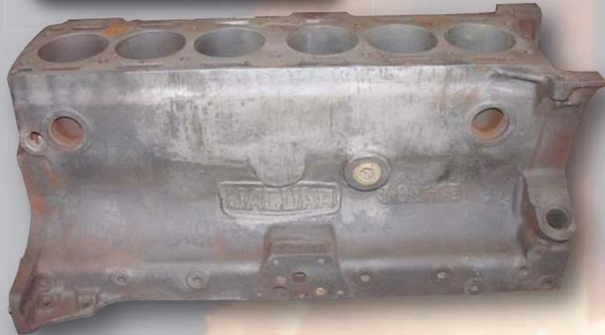
The damaged area was ground out, cleaned up and gas-fusion welded with new metal. The repair was blended in to the original contours and the Jaguar logo rebuilt.
