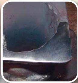
This veteran cylinder/head casting had suffered broken flanges. Both flanges was rebuilt with gas-fusion welding and machined back to standard specification.
