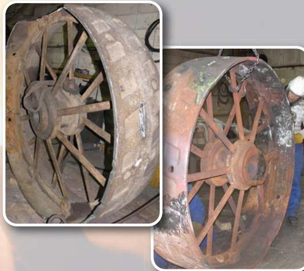
This traction engine wheel has suffered extensive cracking with large sections missing. The internal wrought iron supports were checked and re-welded into place using the gas-fusion process. Patterns were made for casting new sections from material of the same chemical analysis and welded into position.
